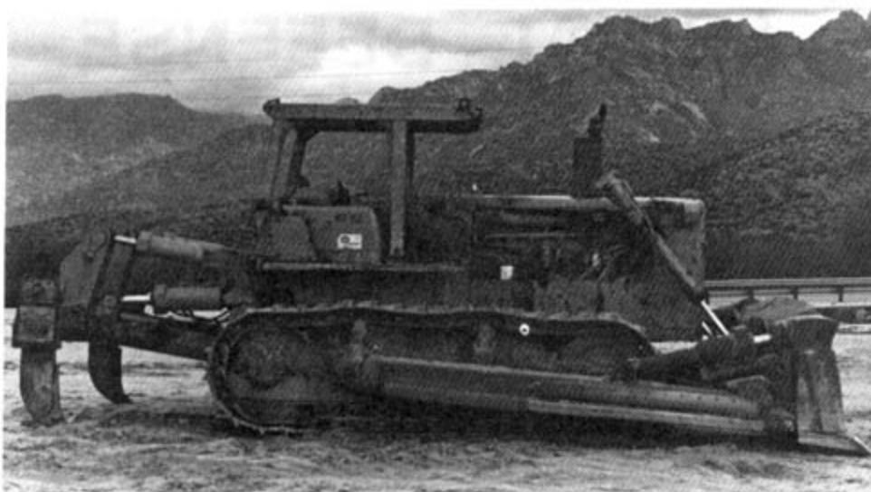
Bulldozer. Note the smoke stack (exhaust pipe).
